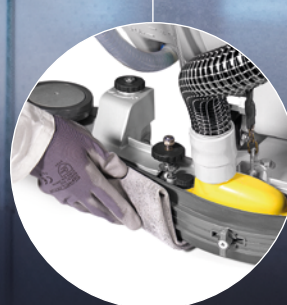
To ensure a perfect drying, the suction hose and the squeegee rubber blades must be cleaned at the end of any cleaning operation. The squeegee can be lifted to quickly clean the rubber blades.
