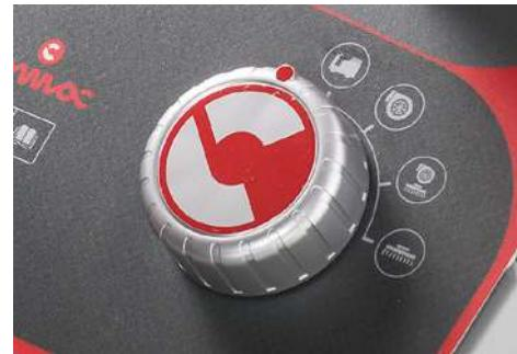
With the working program selector the operator can choose to set the machine operation for: transfer, drying, scrubbing and drying simultaneously or only scrubbing.
