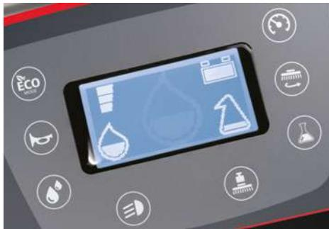
With the versions equipped with CDS dosing system it is possible to be very precise in adjusting water quantity and detergent percentage and to save the settings inside the program selector to use them again automatically for the next cleaning operation.
