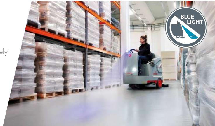
Optima can be equipped with **Blue Safety Spotlight**, the technology that projects a light beam on the ground to indicate the presence of the scrubbing machine in advance, thereby increasing safety
