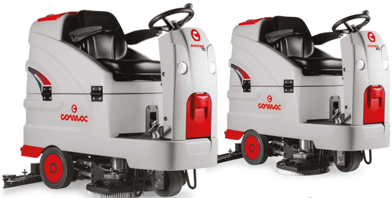
INNOVA COMFORT 75 B Scrubbing version with dual disc brush Working width: 750 mm
