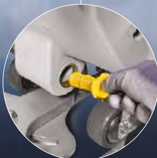
Solution filter cleaning.
